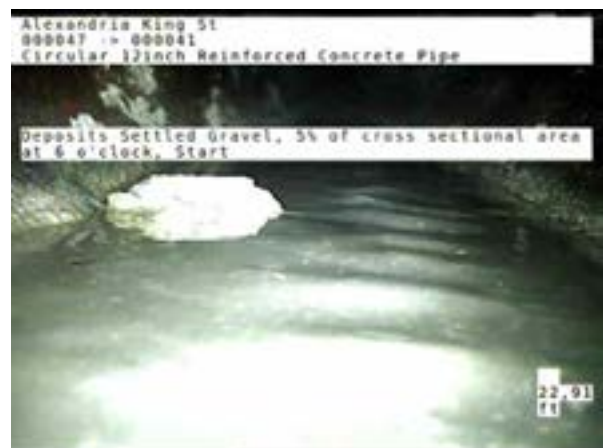
4, 00:02:15, 22.91ft Deposits Settled Gravel, 5% of cross sectional area at 6 o'clock, Start
