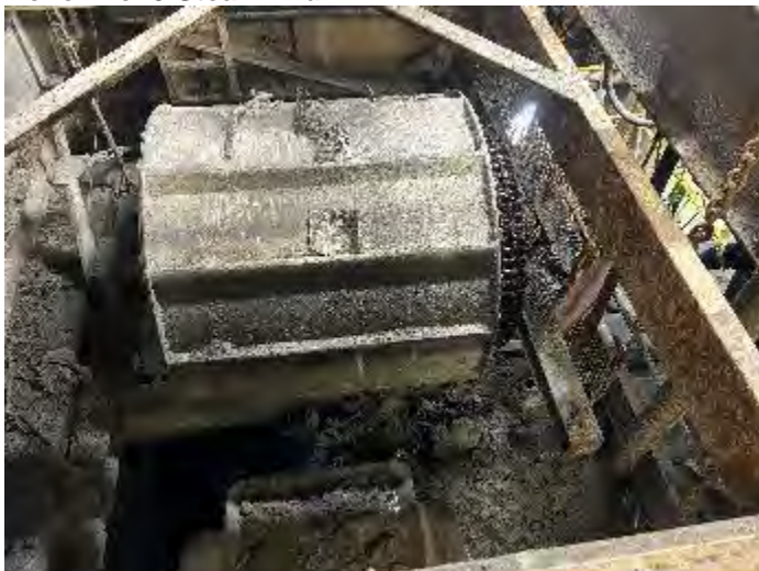
Figure 23: Ferrous drum magnet with ongoing maintenance at the time of HDR site visit
