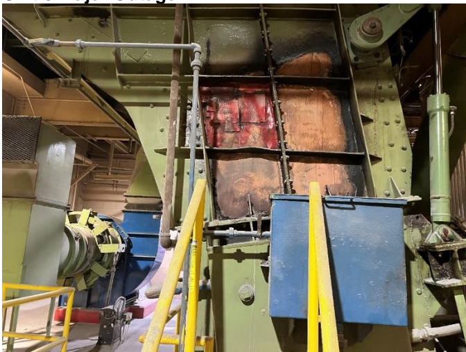
Figure 15: Unit 1 side walls of feed chute in poor condition
