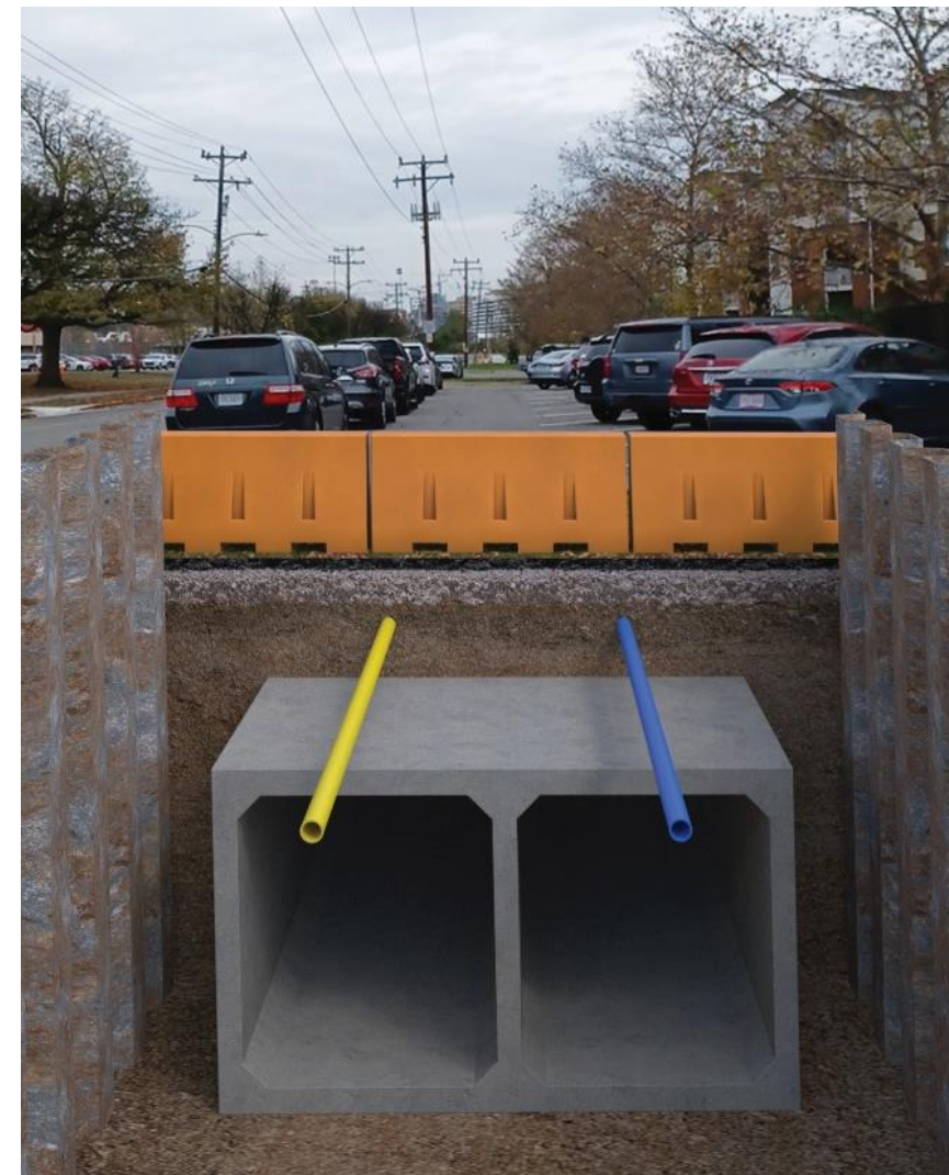
Two 8' x 7' box culverts will be installed on the east side of Commonwealth Ave
