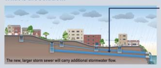
A new and larger-capacity storm sewer will provide an additional route for stormwater to drain. This extra capacity will relieve the existing pipe and mitigate flooding on the road.
