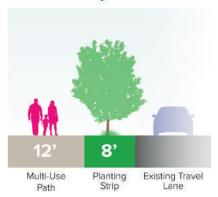
**Primary:** Applies when a cross section is not specified for a street or portion of a street.
