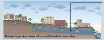
A new and larger-capacity storm sewer will provide an additional route for stormwater to drain. This extra capacity will relieve the existing pipe and mitigate flooding on the road.
