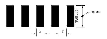
NOTE: CROSSWALK MARKINGS PERPENDICULAR TO VEHICLE WHEEL PATH
