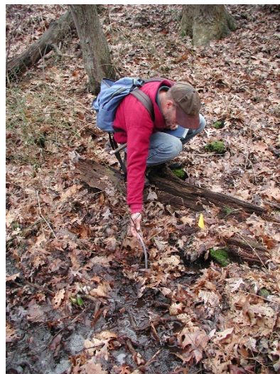
Measuring the flow of groundwater in an Acidic Seepage Swamp with a piezometer.
