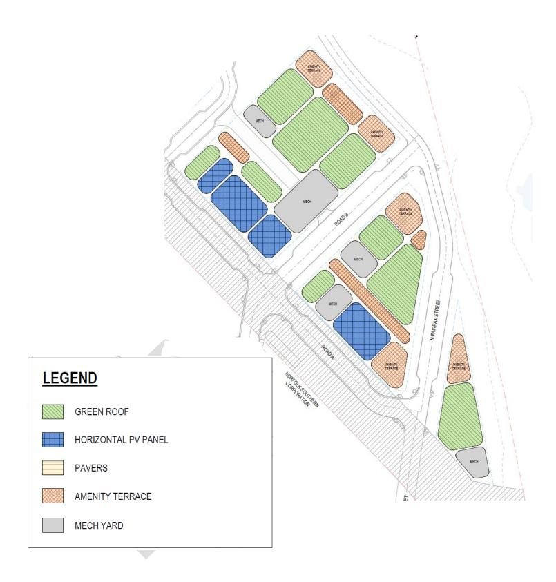
The PRGS team will continue to study the feasibility of incorporating solar PV panels as building massing, orientation, roof area and mechanical penthouse areas are further defined at each Block DSUP.
